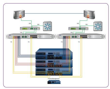
At the very top left and top right are firewalls (shown in red "brick"). On the left is the active firewall; on the is right the standby firewall which enables the High Availability aspect of the solution. At the bottom left and right in light blue are network switches. The diagram shows the Net Optics iBypass 10G Tap connected behind the firewall and network switches.
