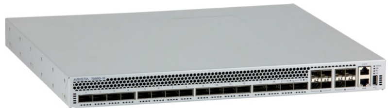
Arista 7050Q-16: 16 x 40GbE QSFP+ and 8 x 10GbE SFP+ ports
