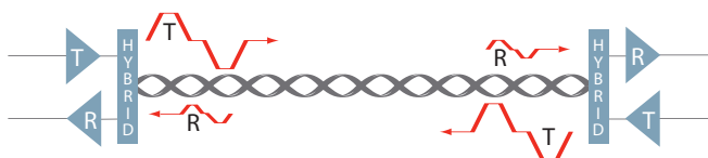
Bidirectional – Transmit and receive on the same wire pair (1000Base-T and 10GBase-T)
